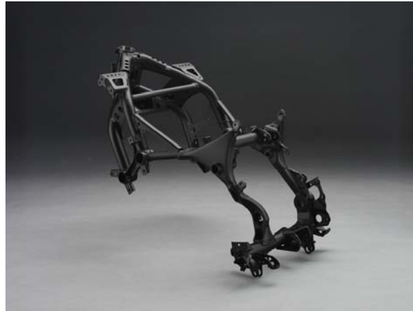
High tensile steel dual backbone frame uses engine as stressed member and allows low mounted fuel tank
