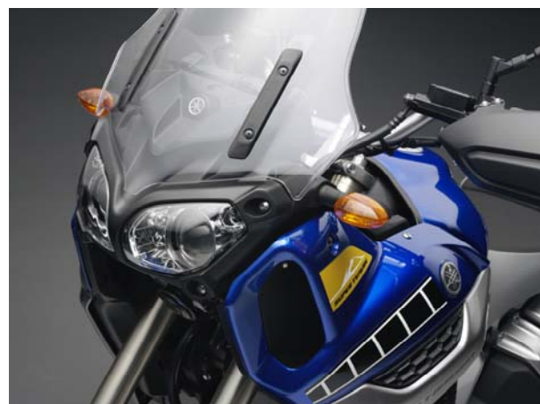
Functional design includes air intake for side mounted radiator and excellent wind protection
