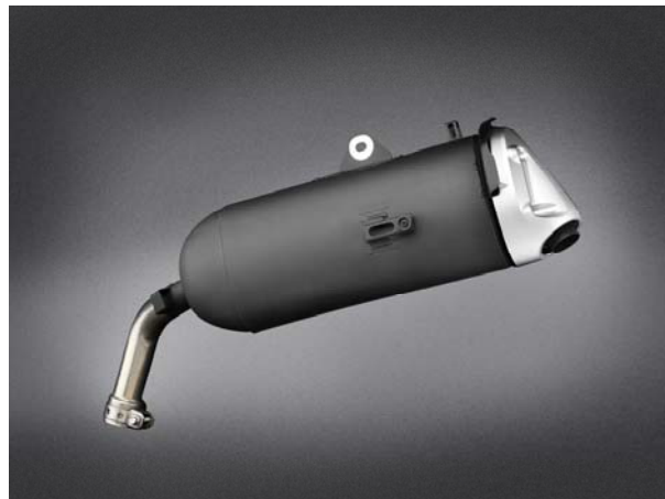
Compact two-into-one muffler meets the most stringent emission laws
