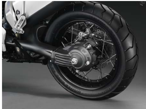
Final drive is via low maintenance shaft that employs a compact hypoid gear for less unsprung weight
